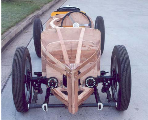
Body frame on chassis complete and ready for skinning.
