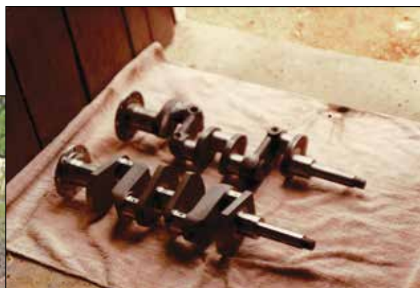
The billet crankshaft (bottom) is much more substantial than the original.
